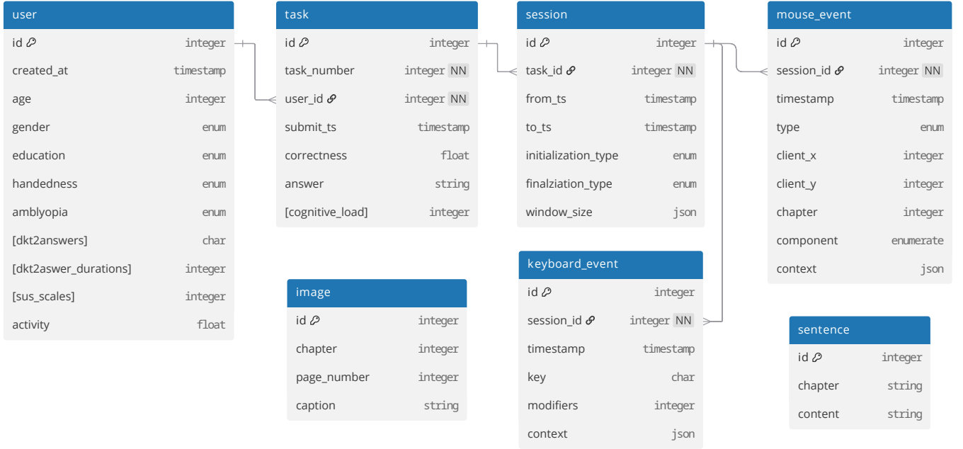
Figure 6: The underlying schema of the GUIDETA. Note, that image and sentence tables are connected to the keyboard_event / mouse_event tables via their context attribute in which the respective IDs appear.
