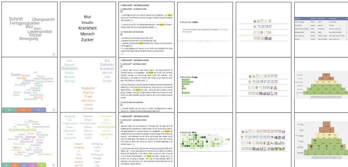
Figure 1: Text visualizations with different LoD in our CHIS. The document is analyzed using Latent Dirichlet Allocation (LDA) applied to its paragraphs. (First column) A word cloud visualizing the most dominant terms across several topics. The size of each word represents its relevance, while the color indicates its associated topic. (Second column) A topic cloud displaying the most relevant terms within each topic, offering a more focused view of the topic structure. (Third column) Text snippets highlighting terms that signify specific topics, providing contextual insights. (Fourth column) A tile bar designed to help users localize terms within the document, offering a compact overview of term frequency and distribution. (Fifth column) Infographic-based visualizations convert important content from the document into graphical representations. Each row corresponds to the different LoDs for each visualization method.
